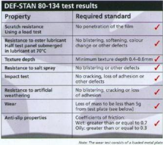
Note: The wear rest consists of a leaded metal place being drawn back and forth in contact with the fast plate at 37 cycles per minute. The wear blade is of mild steel to 853900 part A3 2.1 and, for the purpose of the test, is loaded with a 5000g weight.
